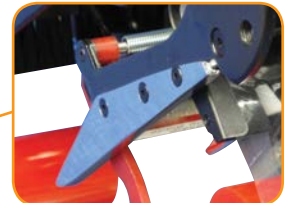
Front and rear tape legs adjustable from 2 to 2.5 inches
