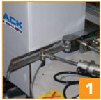
1 Pneumatic arm squares cases before sealing
