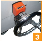
3 Analog counters simplify changeover
