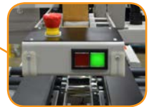
Color coded indicator assures proper spacing between cases
